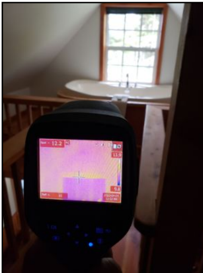
Thermal camera used to check insulation in finished spaces, no voids noted.
